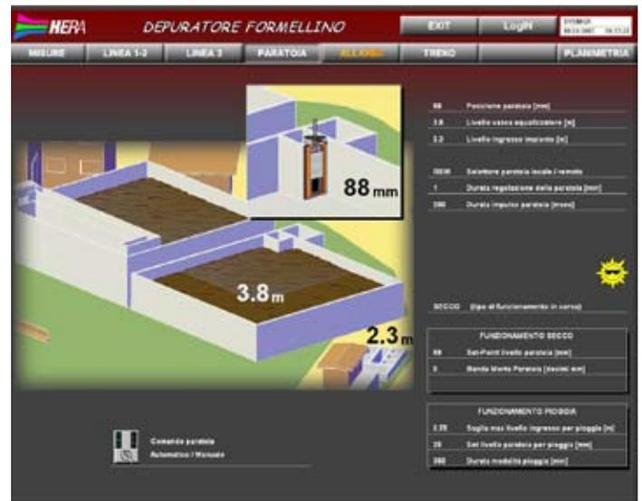
The water flow through the various stations of the water treatment plant is adjusted by controlling sluices.
