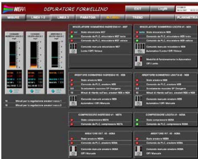
The data collected from the field are used to carry out a predictive control and therefore optimise machine use.
