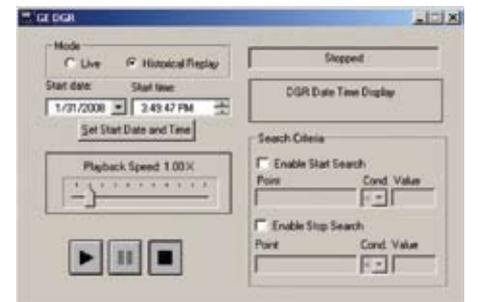
A powerful troubleshooting tool, DGR allows you to playback from a point in time, or you can have the DGR search for conditions in the data and automatically set start and stop times based on those settings to determine the cause of events.
