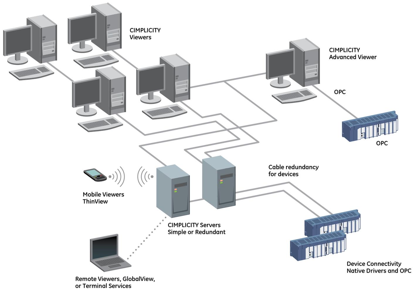
CIMPLICITY is a highly scalable solution that can run in a simple or redundant architecture with a wide variety of viewer or client options to offer flexibility when architecting your solution, providing you with more control over how and where you view your data.
