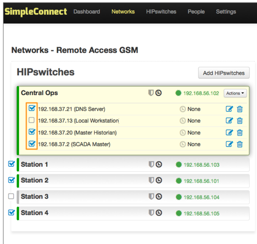
FIGURE 3: SCREENSHOT SHOWING DEVICE-LEVEL POLICY CONFIGURATION FOR A GIVEN HIPSWITCH. (THE ORANGE BOX HAS BEEN ADDED FOR EMPHASIS)
